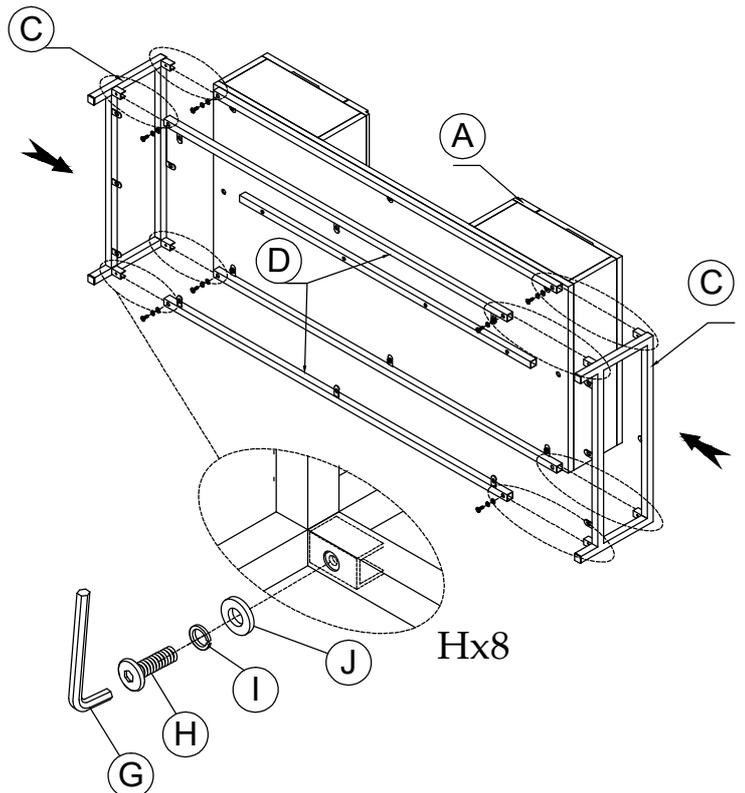
Step 3: Using the Allen key to tighten all bolts
